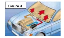
is absorbed by the engine coolant and is circulated using a pump driven by a pulley on the engine. The coolant passes through a heat exchanger where heat is transferred to the driver's compartment using a fan. To eliminate running the engine for heat and coolant circulation an Espar Hydronic 4 coolant heater (see Figure 4) should
